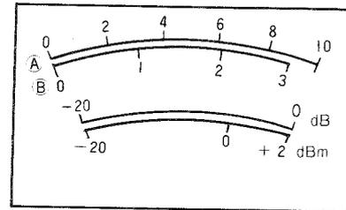
Figure 3 – Meter Scale Graduation
