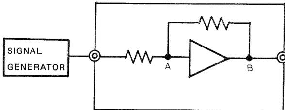
**Figure 5 – Negative Feedback Amplifier Gain Measurement**
