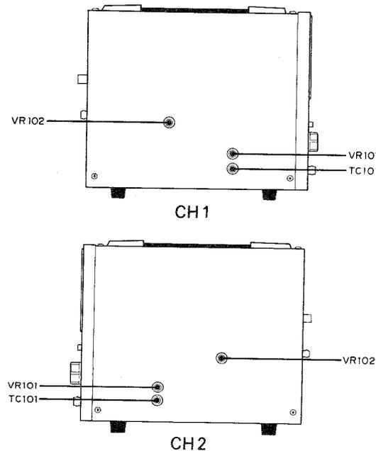
Figure 9 - Pres. Controls on Side Panel
