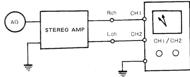
Figure 6 – Stereo Amplifier Frequency Response Measurement
