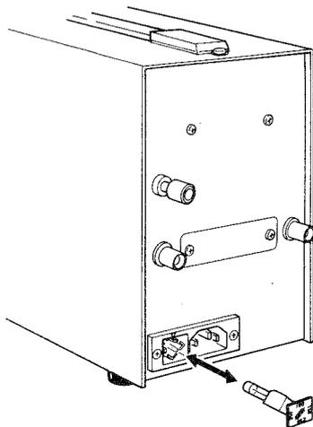
Figure 8 – Replacing the fuse
